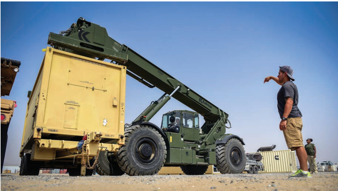
U.S. Army Staff Sgt. Abraham Ruiz, right, a K motor transport operator, helps movements specialist Sgt. William Poley, both with the 117th Combat Sustainment Support Battalion assigned to the Joint Special Operations Forces Support Detachment, use a Kalmar RT240 rough terrain container handler to lift equipment June 4, 2018. JSSD-K operates Camp Sparta, a trans-regional, intermediate-level staging base and logistics hub for special operations personnel.
